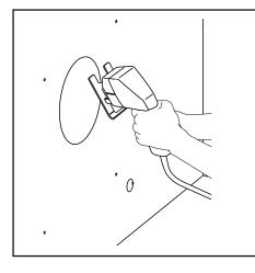
Use a jigsaw to cut the holes out of the wall and discard the inner circle debris. The wall is now prepared for the installation of the unit.
