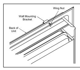
Secure the back of the unit into place using two (2) wing nuts and washers.
