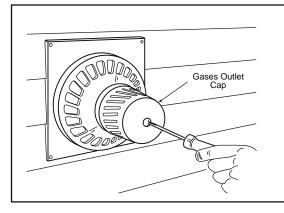
Attach the gases outlet cap making sure that the threaded rod comes through the center hole in the cap. Secure the gases outlet cap by attaching the washers and the brass blind nut to the threaded rod using a screwdriver, tightening to stabilize the vent kit.
