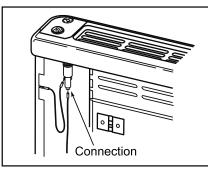
Connect wire from piezo igniter to igniter (arrow). Light the appliance carefully checking all connections with a soapy water solution to assure no leaks are present.
