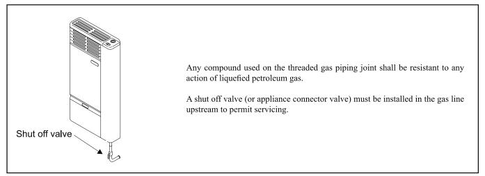
After completion of gas pipe connections, all joints must be checked for gas-tightness by means of leak detector solution, soapy water or an equivalent solution, as applicable.
