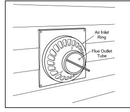
Slide the air inlet ring onto the air inlet tube making sure that the flue outlet tube comes through the center hole to proper length.
